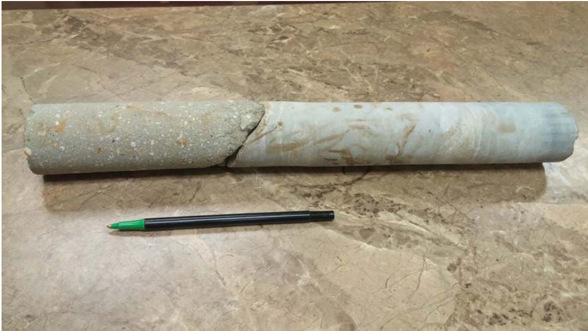
Figure 7. Photo of Rock Core and Grout Encountered in Drilling through Column Locations
